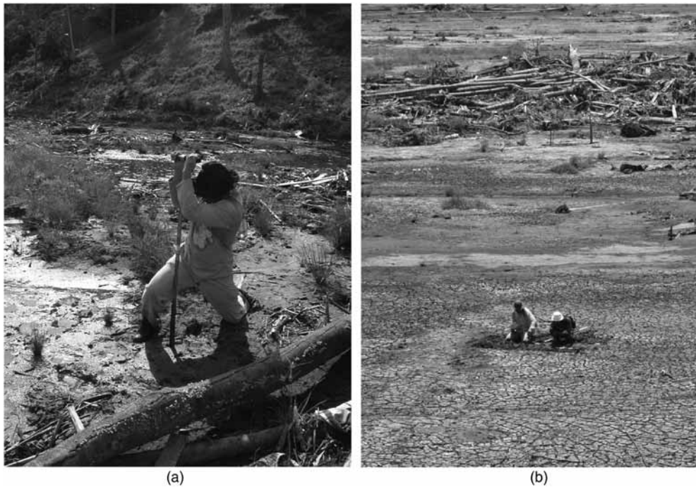
Figure 5. (a) Push coring in search of paleotsunami deposits at Jantang (photo: L. Dengler). (b) ITST members examining a trench in a tsunami deposit approximately 1 km inland at Kuala Meurisi, Sumatra. Note the laterally continuous nature of the deposit, water ponded in local topographic lows, and mud cracks at the surface of the deposit. The trees in the photo were ripped up from a seaward location and transported to this location by the 26 December tsunami. The trunks are oriented parallel to the tsunami flow direction (photo: B. Jaffe).
